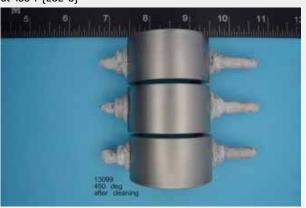
Table 17: Testing for GHSC and SSC were done in accordance with TM0177-2004, method A - Tensile test, in NACE solution  $A^{\Psi}.$  One set of samples was coupled to steel via the stressing bolt and the other set was tested without steel coupling. Applied stress was 90% of actual yield strength.
