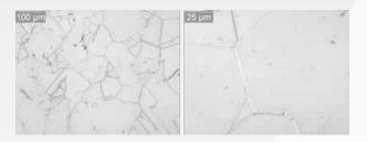
Figure 17: Scanning electron micrographs of 10-inch (254 mm) diameter alloy 945X® rod at center in longitudinal orientation.
