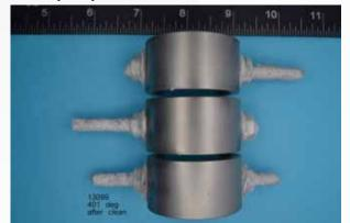
Table 16: C-ring test results in NACE level VI- $450^{\circ}$ F [232°C]. The environmental conditions were as follows: 3.5 MPa [500 psia] H<sub>2</sub>S, 3.5 MPa [500 psia] CO<sub>2</sub>, 20 wt% [139,000 mg/L CI] NaCI, at 232°C [ $450^{\circ}$ F]. The applied stress was 100% of the actual yield stress at temperature.
