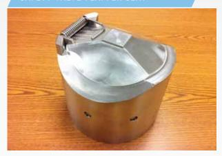
FORGING FOR A TUBING HANGER
