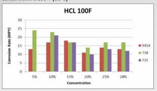
Figure 12: Weight loss of alloys  $945X^{\oplus}$ , 718 and 725 at various HCl concentrations at  $190^{\circ}F$  ( $88^{\circ}C$ )
